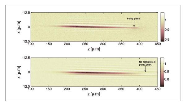
Figure 1: By carefully tuning the probe pulse at the anti-stokes wavelength of the pump pulse, it is possible to detect the pump pulse as an absorption feature of the shadowgram, thanks to an inverse Raman scattering process. The effect is evident from the comparison of the shadowgrams for probe at the anti-stokes (top) and pump (botton) wavelength. In the latter image the signature of the pump pulse is absent (adapted from Minardi et al. 2014).
